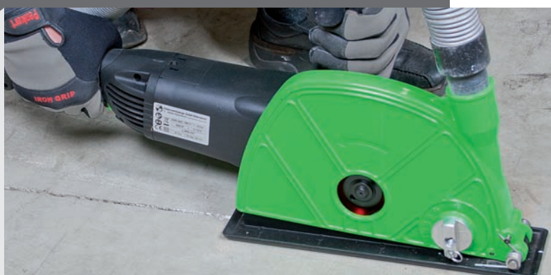
adjustable cutting depth
