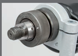
Adjustment ring for soft percussion
