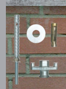
Fastening set brickwork with Rawl-anchor M 12, Ø 20 mm, tightening screw with nut and washer, wing nut, washer
