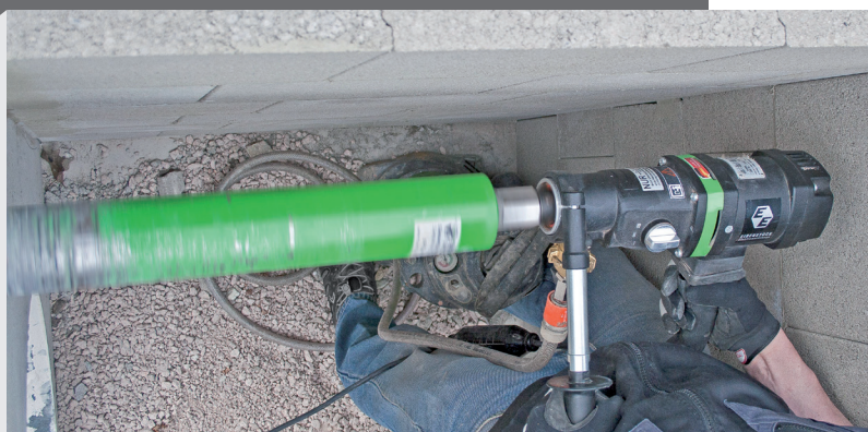
Changing system – water supply and dust extraction
