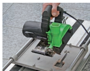
fixing of the saw without any tool
